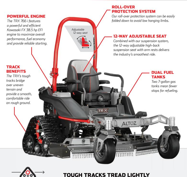
The patented TRX rear torsion axle track system delivers maximum traction for stability and low ground pressure for minimal compaction. All-terrain Tracks follow the contour of the ground and provide a smooth ride. The 11" wide tracks are ideal for side hilling, soft terrain and rough areas other mowers can't reach. Optional Turf Tracks are less aggressive and perfect for soft ground, rolling hills and sensitive terrain.
