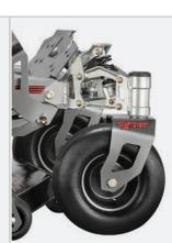
The Altoz Independent Front Suspension (IFS) smooths out rough terrain for superb comfort and control. Available as an accessory on TRX 354 models.
